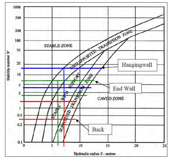
Figure 16-11: Stability Graph Method (Bawden 2005)
