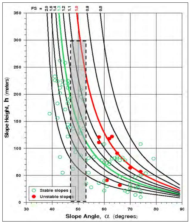
Figure 16-5: Slope Height by Slope Angle – Factor of Safety (Hoek & Bray, 1974)
