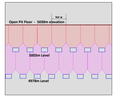
Figure 16-39: Typical Long Section of SLC Stoping Immediately Below Open Pit Floor
