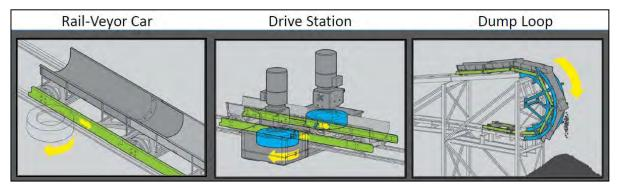
Figure 16-34: Rail-Veyor Shuttle System Operation
