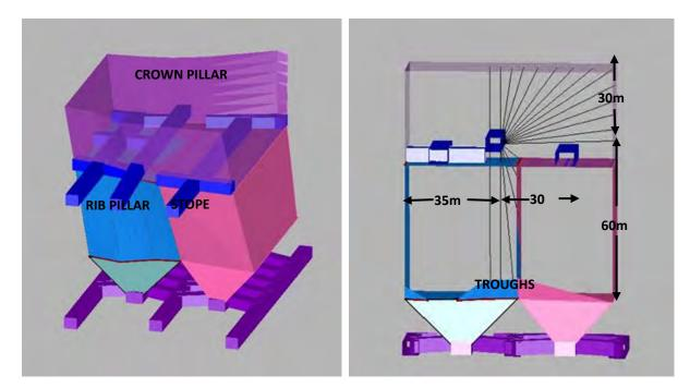
Figure 16-37: Slot and Mass Blast Stope Design
