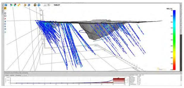
Figure 16-4: Troilus Project RQD Values by Drill Hole
