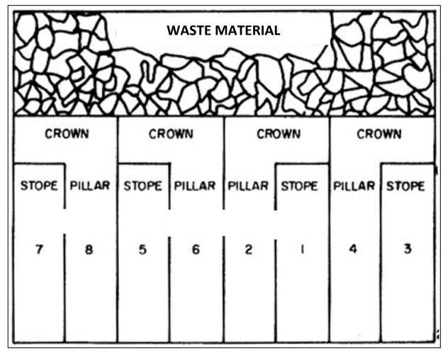
Figure 16-36: Illustrative Long Section of the Slot and Mass Blast Method
