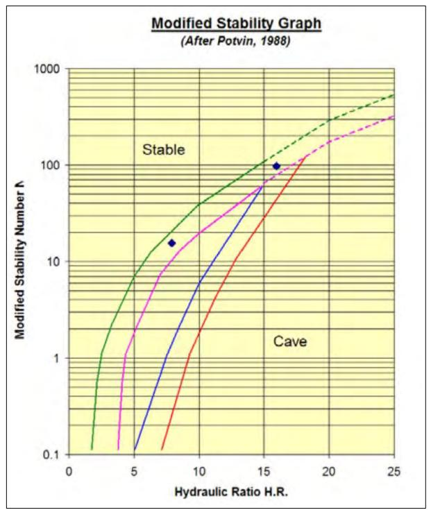
Figure 16-12: Modified Stability Graph Method (Itasca 2006)
