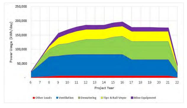
Figure 16-51: Power Usage Rate
