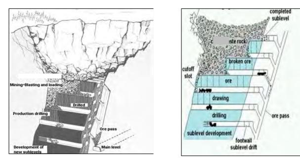
Figure 16-38: Typical SLC Stoping Operations
