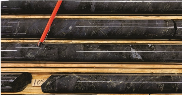
High grade Au-Cu mineralization hosted in magnetite-rich, silicified breccia in hole TLG-ZSW20-184. Gold is hosted in chalcopyrite-pyrite stockwork fracturing. Local sulfide concentration along foliation plan. Biotite-rich.
