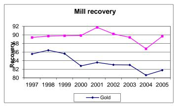
The results highlight the impact of grind on gold recovery, and hence within the flowsheet recommended by this study a finer grind ( $80\% -75 \mu m$ ) has been selected. This should help to obtain the 90% gold recovery targets used in the current work.
